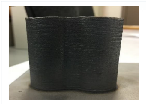
Figure 1: Single Wall Dumbbell Structure Fabricated from Stainless Steel 420LC
