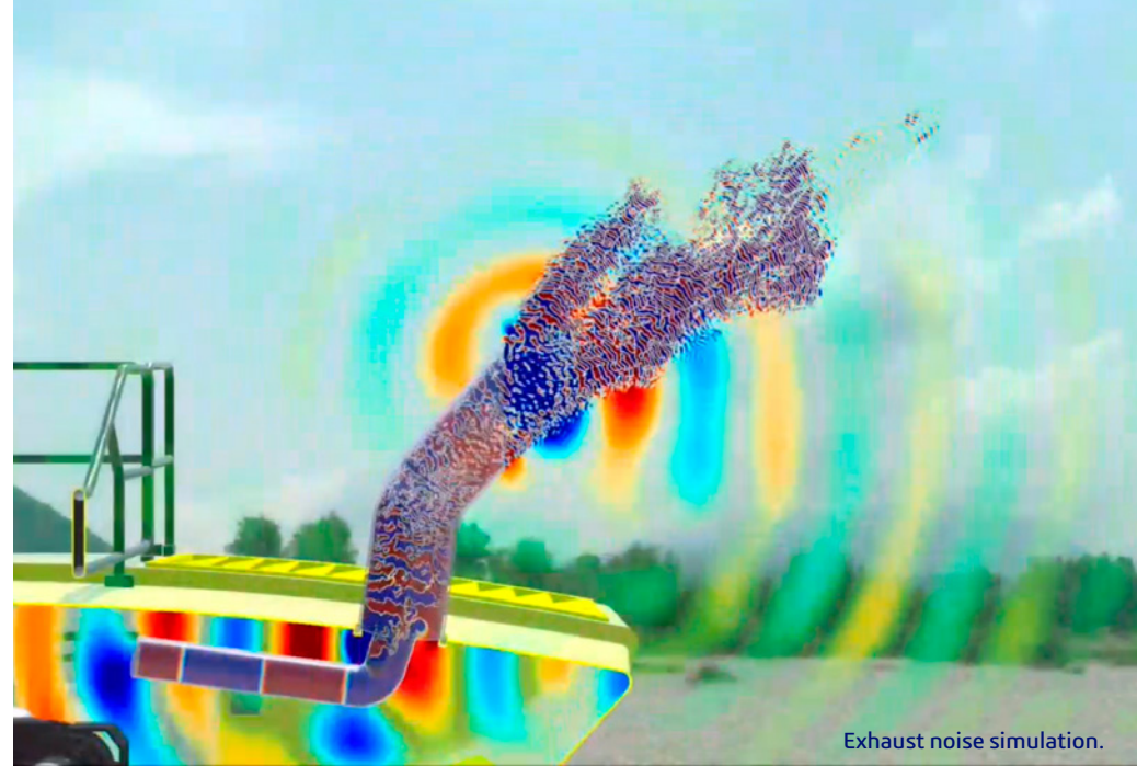
Total Noise Simulation, including simulated fan noise, simulated exhaust noise, and measured engine noise.
