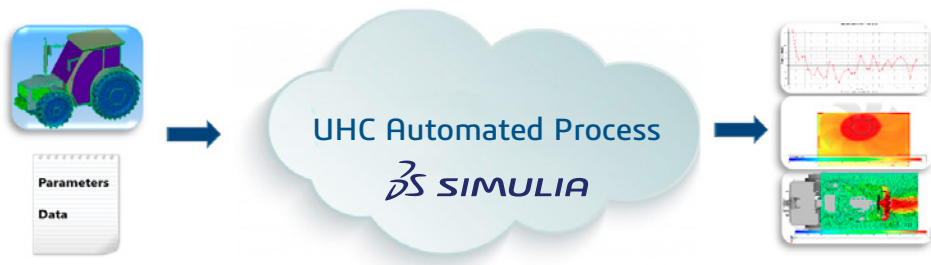
SIMULIA-Cloud Underhood Cooling Automated Process.
